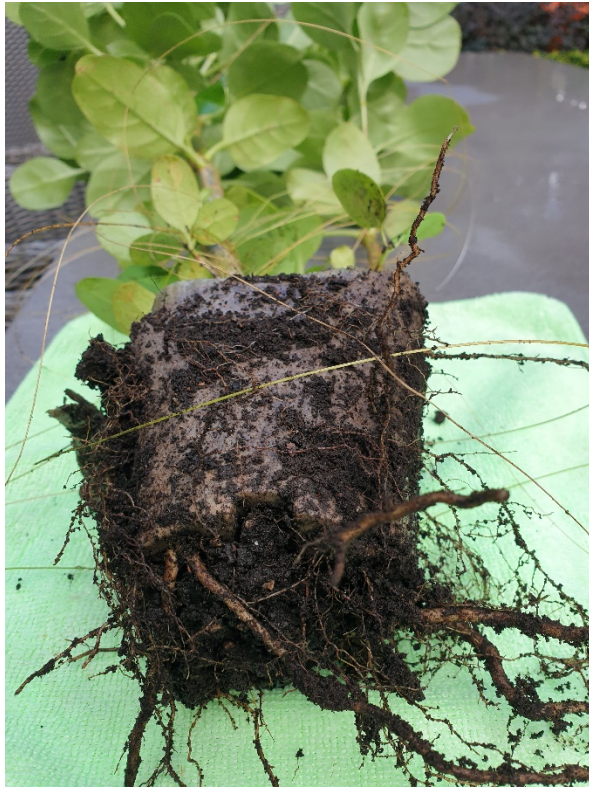
Image 3 After 6 Months in Soil Compostify Pot is Biodegrading and Plants Roots Penetrating Pot Base
